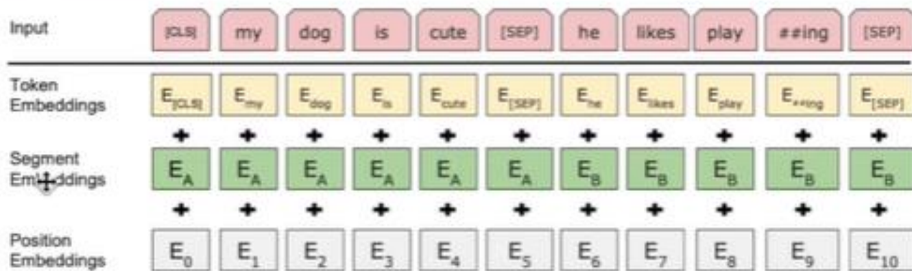
Figure 2: BERT input representation. The input embeddings are the sum of the token embeddings, the segmentation embeddings and the position embeddings.
